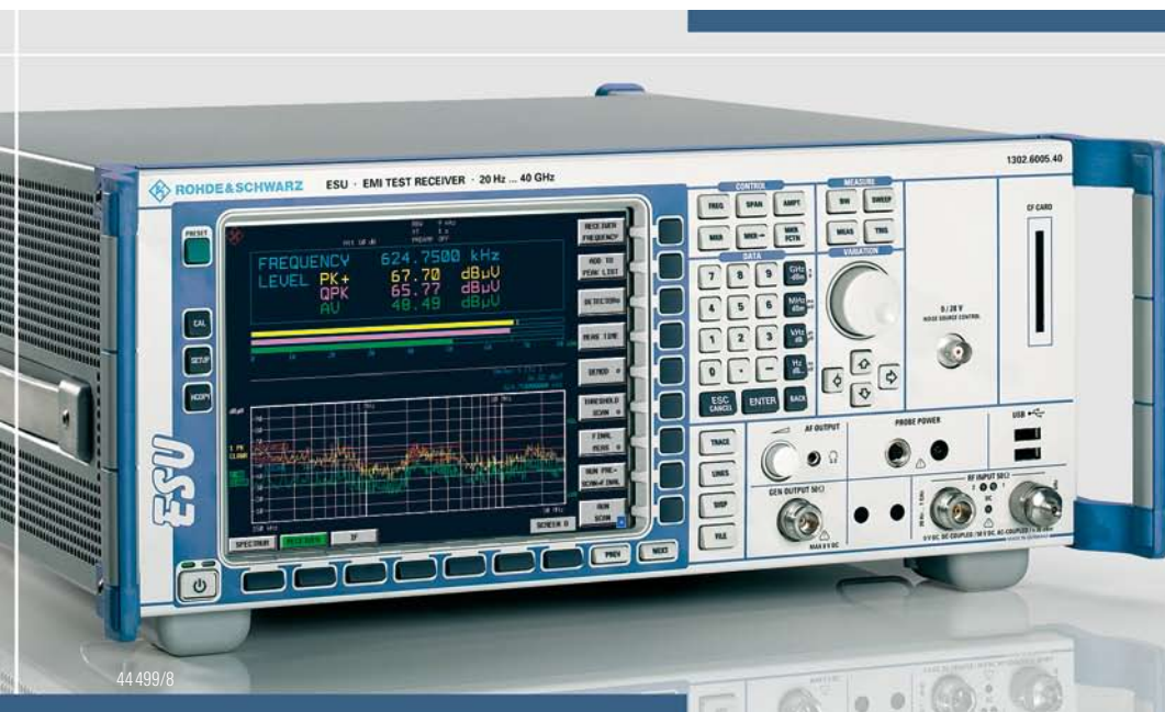
FIG 1 Above 3.6 GHz, the measurement sensitivity of the R&S®ESU EMI test receivers can now be significantly increased by adding the new preamplifiers.
